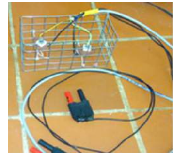
Fig. 2: fix the sensors in metal basket at different depths
