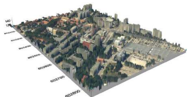
12. Figure 3-dimensional urban model, applied of LIDAR data (0,5 m) and high resolution true orthophoto (~0,2m), Székesfehérvár
