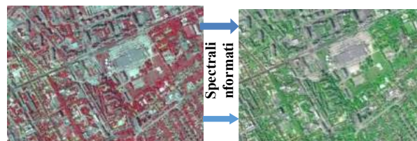
3. Figure True colour and false colour orthophoto of Székesfehérvár based on aerial images
