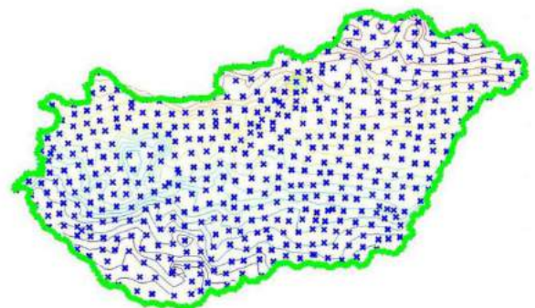
Figure 6. The point distribution of the MGH-50 gravimetric network
