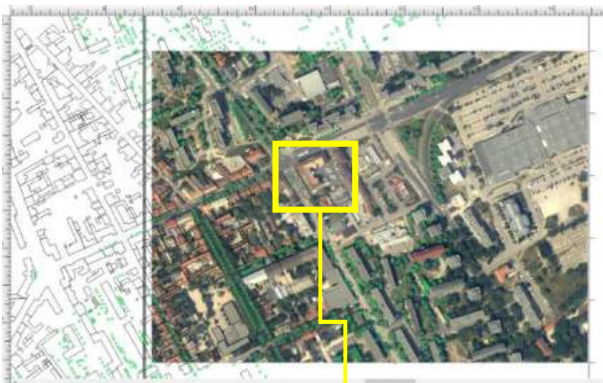
15. Figure Cadastral map, high resolution true ortho photo and depicted individually measured trees in a common reference system
