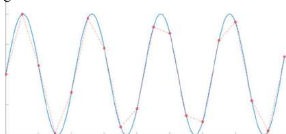
Figure 1. Sampled signal is approximated by linear interpolation.
