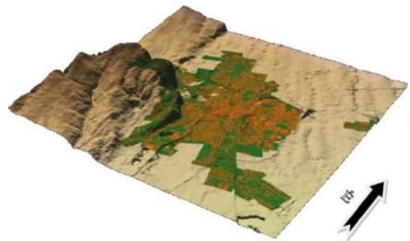
10. Figure Green and artificial land cover, classified satellite image draped on DTM (20m grid size) [10]
